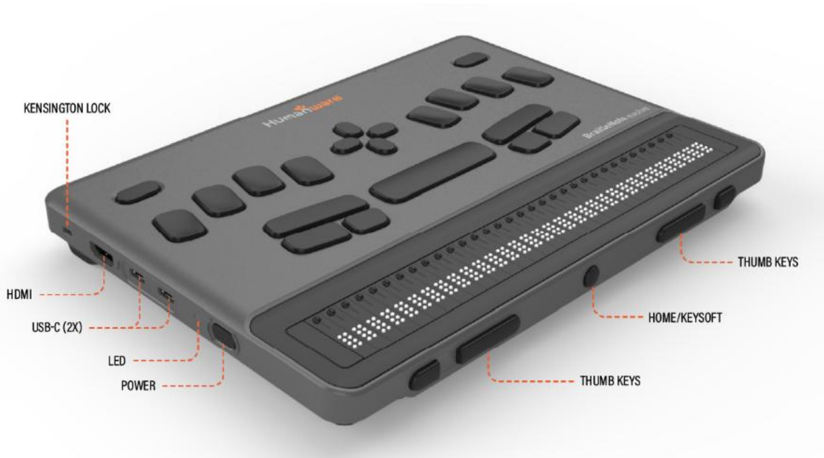
Fig 2 – Image of the BrailleNote evolve left side edge indicating the ports and buttons on the left side and the front edge.
